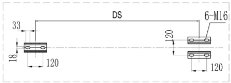
Location Plan of Anchors (DS is the distance between the front leg and rear leg)
