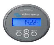
The essential function of the battery monitor is to calculate ampere-hours consumed and the state of charge of a battery SOC. Ampere-hours consumed is calculated by comparing the current flowing in or out of the battery.
