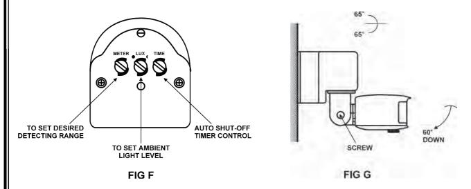
Turning the switch OFF will turn off the sensor and the controlled unit. When switching the power switch ON, the sensor will automatically switch ON (in AUTOMATIC MODE). Leave the power switch ON for normal operation. The sensor will either switch the light on at night or the whole day – depending on the setting of the daylight sensor. (LUX)
