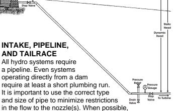
pipelines should be buried; this stabilizes the line, reduces accidental damage and prevents animals from chewing it. Put markers down at regular intervals to alert anybody to the fact that there is a buried water line and not to start digging there without taking appropriate action to prevent pipe damage and unwanted water loss.
