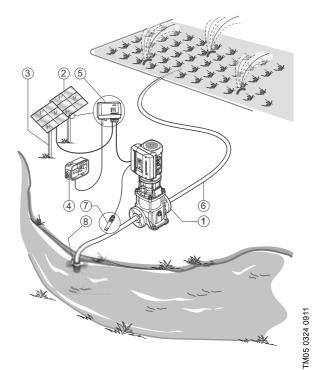
Fig. 15 CRFlex Solar with generator
