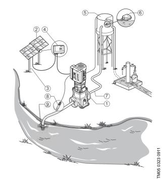
Fig. 14 CRFlex Solar with level switch
