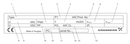
Fig. 1 Nameplate of the MGFlex motor
