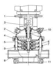
Fig. 12 Sectional drawing of CRFlex pump end
