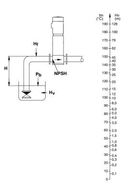
Fig. 10 Minimum inlet pressure - NPSH
