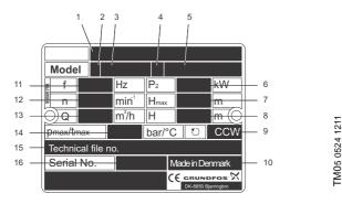
Fig. 9 Nameplate of CRFlex pump end
