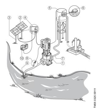
Fig. 16 CRFlex Solar with level switch and generator
