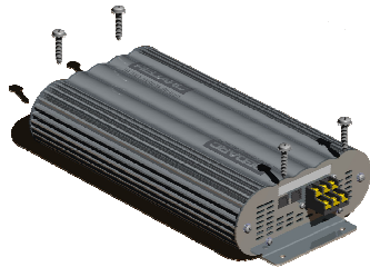
Figure 2.2.1.1 – Horizontal mounting: acceptable
