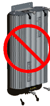
Figure 2.2.1.3 – Do NOT mount the unit this way
