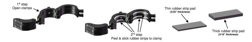
c) Attach the clamps to the roll-cage as shown below and pre-adjust tightening tension of all clamps. NOTE: Keep all clamp handles open as shown in step 3 below; this will allow you to move the clamps up or down when installing the windshield for the first time.
