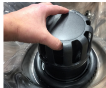
Pull Up to Remove Floater Assembly
