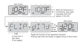
**Note:** Some panels may have a dedicated FLIP button, which allows the user to flip the display with a single button-press.
