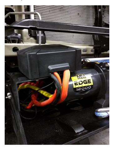
While we used a Mean Mother winch in this photo to illustrate the bracket please note that the control box on Mean Mother winches can mount over the motor side of the winch using factory supplied brackets.
