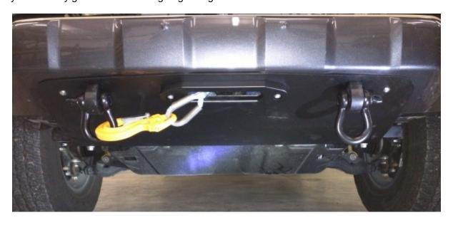
Remove your lower spoiler if your Tacoma included one from the factory. You will not be able to use it with our winch mount. Get out your 4" grinder with a cutoff blade so you can remove the recovery hoop on the driver's side frame horn. You must remove this or you will not be able to install the skid plate. You will create an abundance of sparks so make sure no flammable materials are nearby. **Always** wear safety glasses while cutting! You can paint the end of your cuts to prevent rust.
