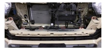
**Step 6**: Remove the 'air dividers' on each side, just inside of the headlights by removing the flush plastic clips and gently pulling away. Twist inwards towards the centerline of the truck to help remove.
