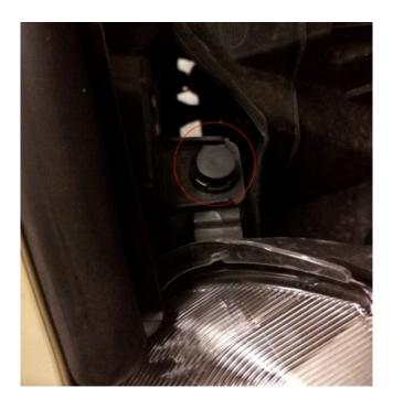
**Step 4**: Use a ratchet and 10mm socket to remove 2 bolts from top of grill. You can now remove the grille by pulling forward and lifting gently.
