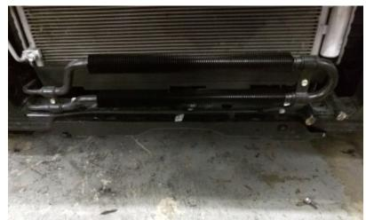
Let's start by removing this bolt on the passenger side on the frame. This bolt mounts a bracket for the power steering line. We need to remove this bolt so the line can move back with the cooler. You do not need to replace this bolt and there is no need for the bracket.
