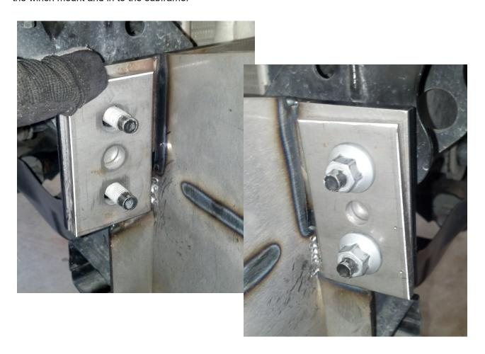
Once the bolts are installed and snug you can tighten the 6 14mm bolts and torque to 40lbs. Tighten the 2 lower bolts and torque to 60lbs.
