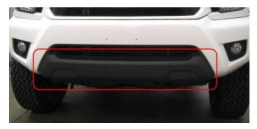
Once exposed by removing the valance you need to cut out the center section so it will fit the winch mount properly. A 4" grinder with a cutoff disc is probably the best method. Take your time and be careful. **Don't cut just yet...keep reading!**
