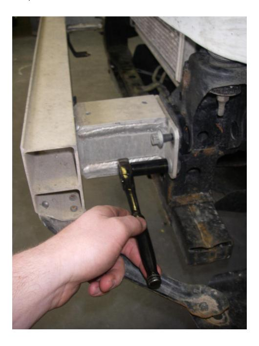
Next you need to remove the two 19mm bolts that hold the subframe ends in place. Leave the subframe ends (they simply slide out but you need them where they are. These two bolts will be used to secure the bottom of the winch mount. Set the bolts aside until you install the winch mount.
