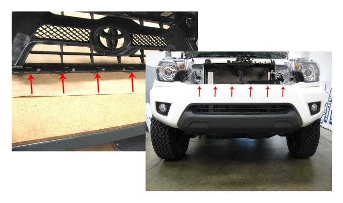
**Step 3**: Remove the plastic clips along the top side of the bumper cover.
