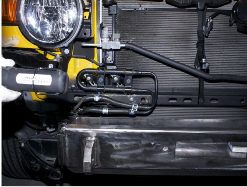
Figure 3: Relocated P/S fluid cooler
