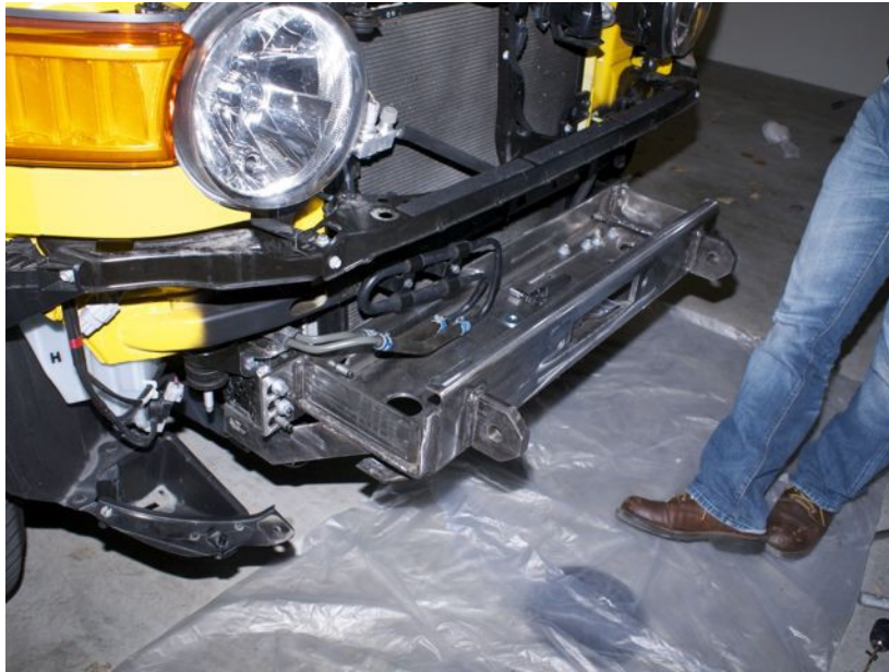
Figure 1: P/S fluid cooler before modification
