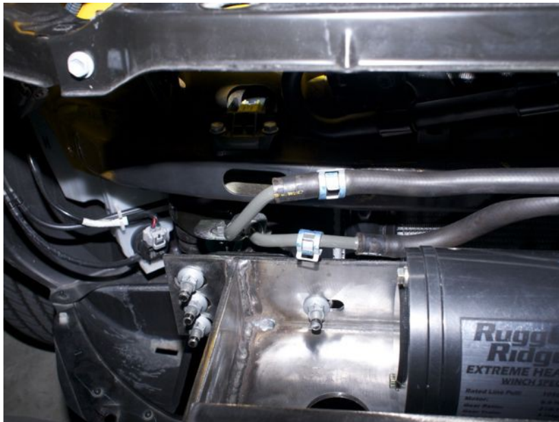
Figure 2: Reshaped pipes with hoses pushed in deeper
