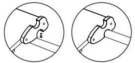
To ensure a safe and stable connection between separate Pikler units, check that each connector hook is fitted securely over a rung and does not shift around.
