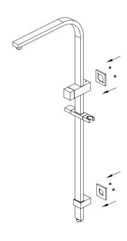
3. Screw the straight tube (with lower body) on diverter body, and then pull on the 2 dressing rings for both the diverter body and lower body.
