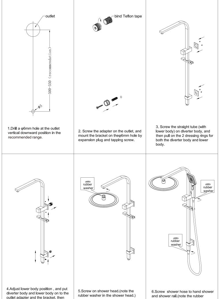
tighten grub screws by Allen key.
