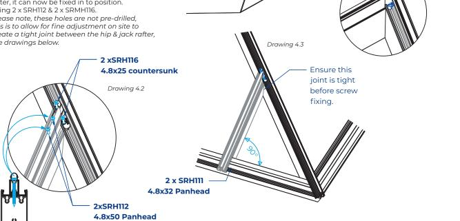
13. Once all the roof bars have been fully fastened to the eaves beam & ridge, you can fasten the roof to the timber upstand, using SRH113 (5.5x70mm) fixings through the pre-drilled holes in the eaves beam. Ensuring the outermost leg of the eaves beam is flush with external upstand. see drawings below.
