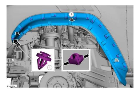
**Step 6:** Remove the vent clips and the fender vent.
