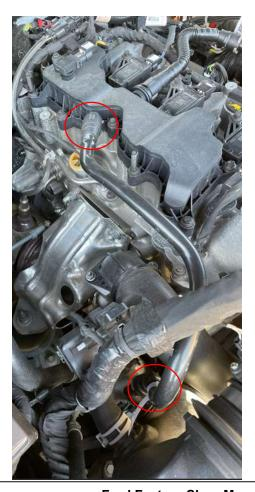
Starting with the passenger side (RH side), remove the existing RH PCV tube. Remove threading pushpins from cowl cover, install RH bracket, and install new 8mm pushpins.
