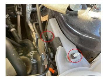
Position bracket as shown and install pushpin through bracket into existing hole in strut tower (just below brake lines). Install M6 locking nut onto coolant reservoir studbolt and torque to 8Nm or 71 in\*lbf.
