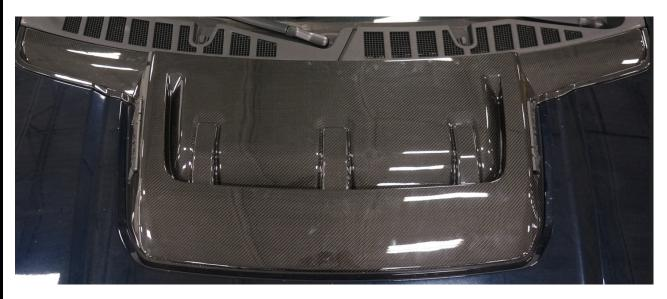
11. Install the supplied 6 Scoop nuts, original 4 nut covers and hood insulation.
