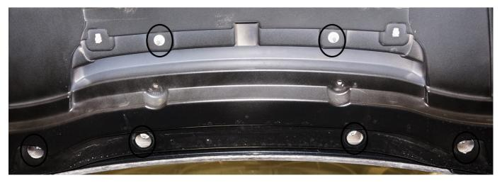
5. Compress retention clips where there is accessibility. Use non-marring tools to pry up the scoop starting from a back corner working around to the front and the opposite side.
