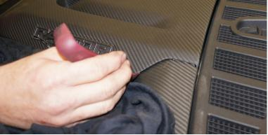
6. Once the front is lifted, use a razor blade to cut the adhesive tape.
