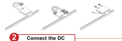
Plug in the MC4 terminals to DC socket on MI
