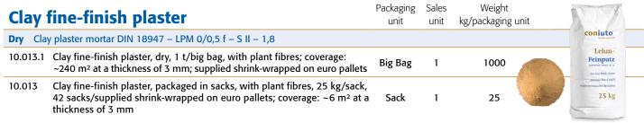
Clay fine-finish plaster is applied at thickness of 1 - 3 mm and skimmed flat or rubbed with a float. It consists of clay-rich earth, fine grain sand > 5 mm and fine organic fibres. It is suitable for machine processing in closed plastering machines, e.g. mixing pump types G4 and G5 or similar.
