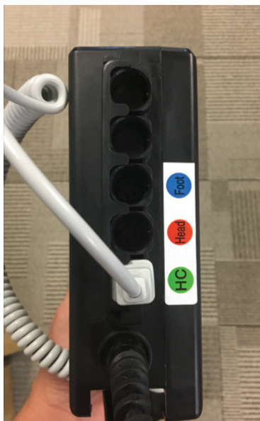
Figure 13: Junction Box, Semi-electric bed
