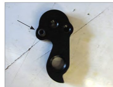
Figure 2 - Setscrew placement for vertical dropouts
