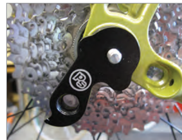
Figure 4 - Mounting for vertical dropouts
