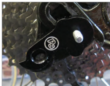
Figure 3 - Mounting for horizontal dropouts
