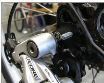
Figure 5 - Universal Hanger with derailleur installed
