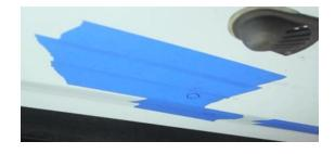
Make sure the masking tape extends at least 6 inches in each direction beyond the marked location. This will help protect the gel coat.
