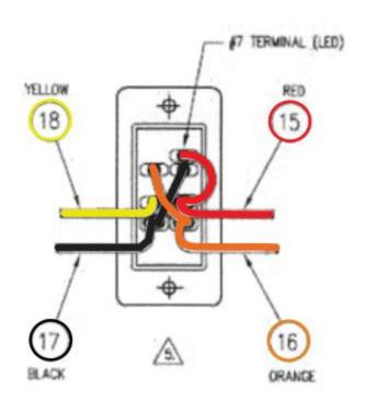
\*\*\* TEST SWITCH AFTER INSTALLING If pump fills when switch is set to empty swap the orange and black wires
