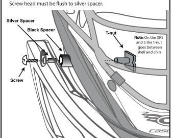
All pieces must be installed for the TPS to work properly.
