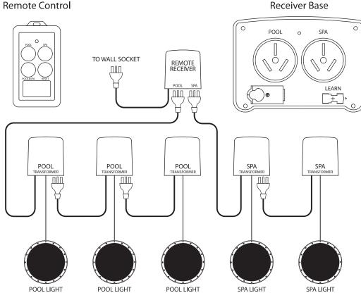
Example Connection Diagram showing multiple light connection
