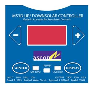
Between the finish time and 8am the unit will display Nop while The unit is not operating pump.
