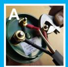
Bolted down connection: please ensure leads and connectors are in good condition and bolted down firmly.
