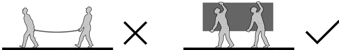
Figure 1.14 – Manutention des panneaux Viroc
