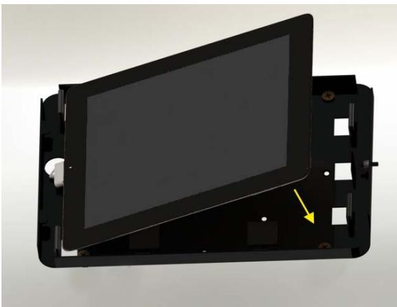
4. If a charger cable is required, connect it to the iPad. Carefully inset the iPad into the bracket at an angle, and push it flat into the bracket.
