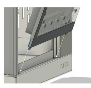
**Step 2:** Now the distroplate is pressed onto the case and fastened with two screws. (Max 3-5 N/m).
