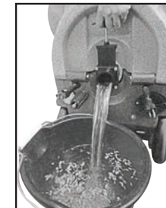
Drain Recovery Tank
