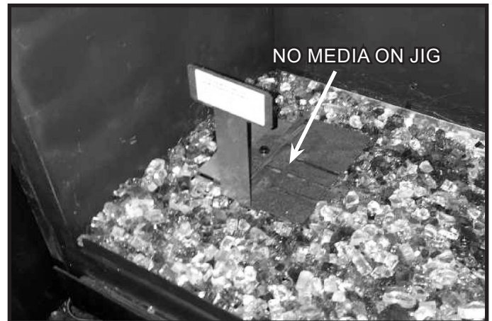
Figure 2. Media Placement Jig in Place
