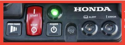
The rammer control panel offers simple startup and speed controls along with LED warning indicators.
