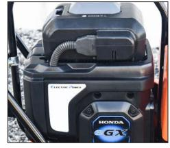
**Honda eGX motors** are fully sealed for protection from dirt and dust.
