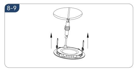
B Place the J-BOX through the cut-out hole and mount according to your local electrical code compliance.
