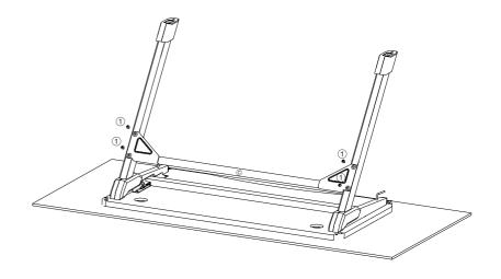
Step 3 Tighten foot pad 2 to connect the legs
