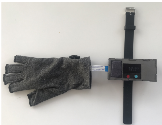
Figure 4: The assembled glove, flexible PCB and hard enclosure
