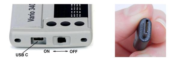
On the left side of Vario 340 you can find the USB port, which is USB type C. Special about the USB Type C port is, that it doesn't matter which direction the USB plug is facing. No more finding the right position of the plug.
