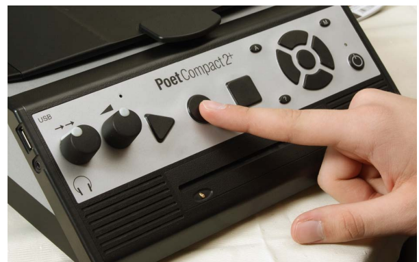
Reading by means of one-touch operation – with 2 buttons or with 3 buttons and menu keypad.
