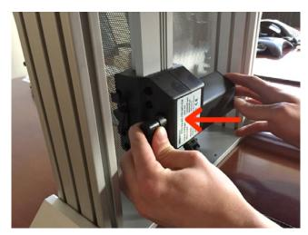
**Step 14:** Route the power cable (C) coming from the actuator motor out the back of the unit through the notch in the back cover and attach the power cord extension.
