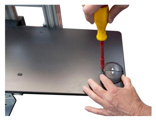
**Step 13:** Plug the connector from the switch located on the top worksurface to the port on the left side of the actuator motor as shown below.
