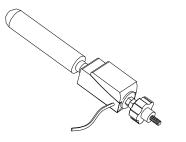
A swiping motion in any direction of the wand activates the switch. This is one of the more universal switches as it can be activated in multiple ways.
