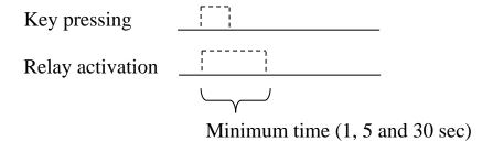
**Maximum time** = Maximum time the relay is activated, then you have to re-activate the relay with the IR-transmitter. Various times can be set.
