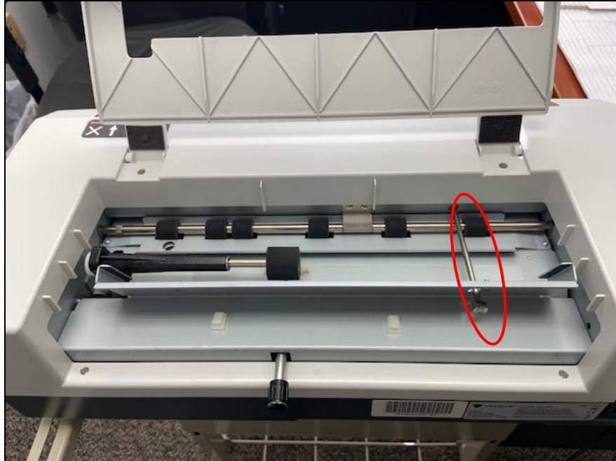
Shows shipping lockout rod to be removed Also note the Paper Feed Adjustment Knob is in place
