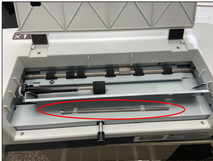
Shows storage area of shipping lockout rod
