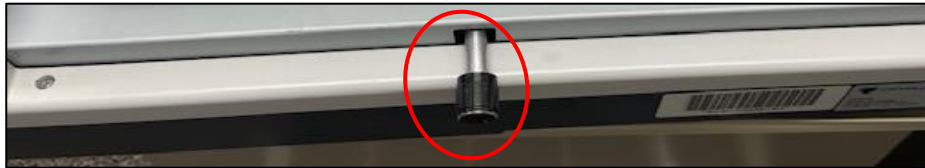
Shows the Paper Feed Adjustment Knob correctly in place
