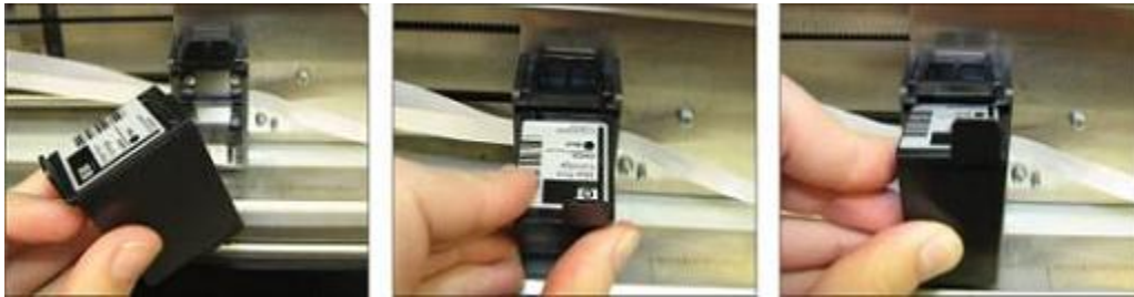
Shows how to insert an ink cartridge
