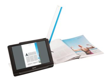
When using Text-to-Speech on a full page, open the camera arm and place the document below the camera. Align the bottom left corner of the document with the blue indicator at the base of the Compact 10 HD Speech.
