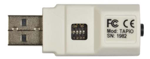
(Tapio mode selection DIP switch. Shown with all switches ON or UP.)
