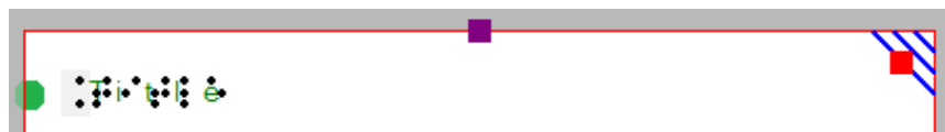
Figure 1. The top of the design shows the title text label, right-up marker and red border for paper size and orientation.
