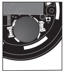
Remove the 3 screws from the underside of the unit and remove the base cover. Fit one 3V Coin Cell CR2032 battery, noting that the '+' terminal goes uppermost (i.e. '+' sign visible once installed). Replace the base cover and fix with the screws.
