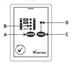
You can pair up to six wireless switches with **CONTROL**, allowing collaboration between several users. If you attempt to pair a seventh switch, the switch that was used least recently will be replaced with the new one. The other switches are unaffected.
