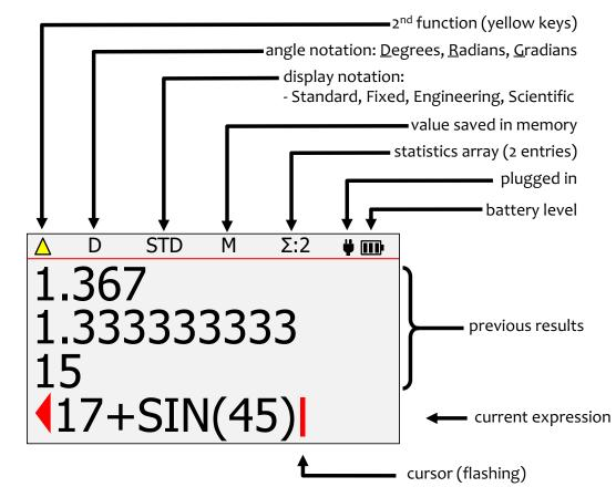
The characters above the horizontal red line at the top of the screen show the *status line* of the calculator. If the battery symbol is animated, this indicates that the battery is being charged. Some of the characters in the status line may not appear at all times. For example, if there is no entry in memory, or if the statistics register is currently empty, these items will not appear.
